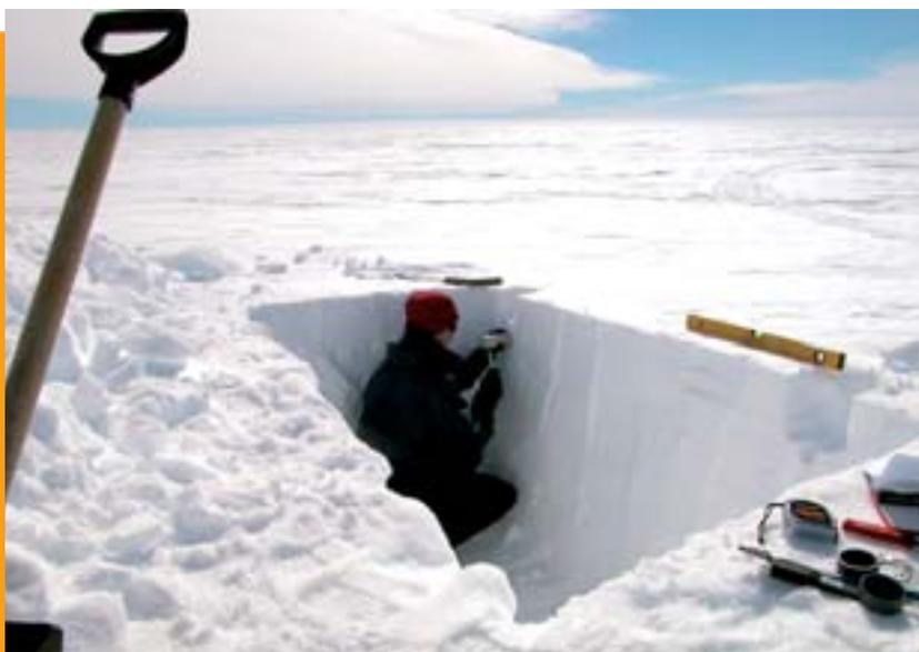
Measuring the physical properties of surface snow in Antarctica.
